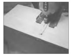
**PHOTO 3:** Opening the rear port after the box is assembled.
