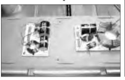
PHOTO 10: Crossovers were pre-mounted on the back panel prior to box assembly, then removed prior to the gluing. This eases later crossover installation.
