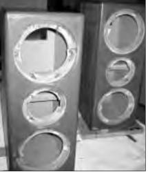
meter. I used 40 grammes **PHOTO 13:** Second primer coat is complete, all of high loft quilting in mounting inserts covered by masking tape.
