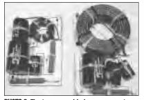
PHOTO 8: The two assembled crossover networks, HF on the left, LF on the right, Components are held in place with cable ties. Stud terminals are press-fit into the 1/8" Masonite.
