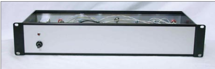
PHOTO 1: Modified Simon amp front panel. Just the power switch and power-on LED.
