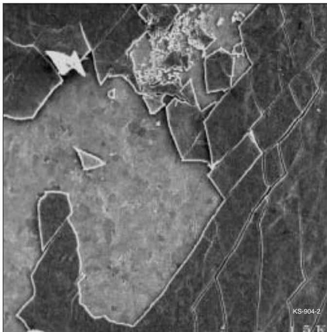
FIGURE 2: SEM image of 1" cone surface showing flaking coating and material underneath.
