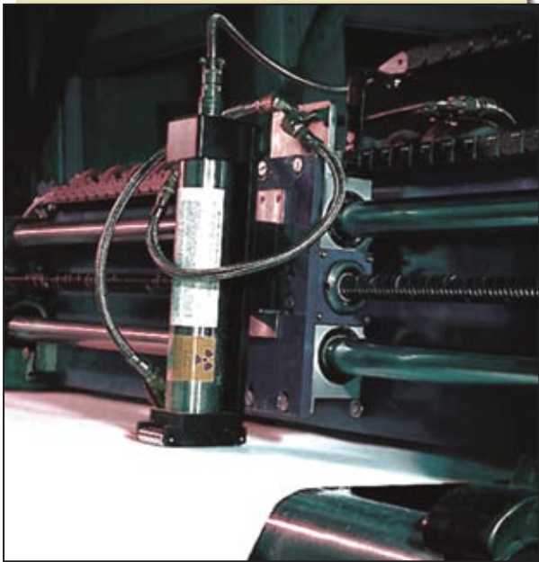
PHOTO 2: Gamma gauge monitoring the quality of the paper as it comes off the paper machine.
