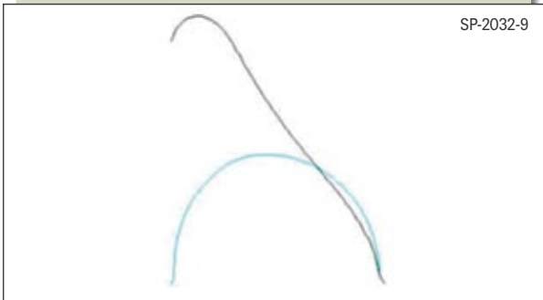
FIGURE 9: Static and displaced shape in the positive y-direction of the 1.0mm thick Arnitel surround.
