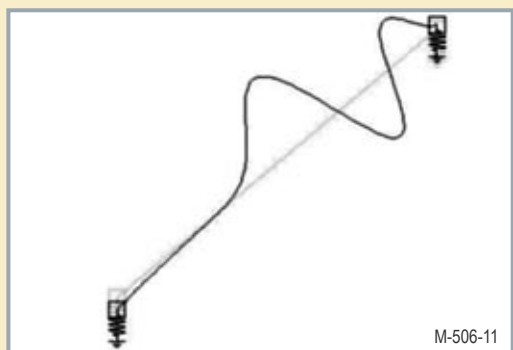
FIGURE 11: Anodized magnesium cone mode shape at f_3 = 1.93\text{kHz} , modal damping = 0.005.
