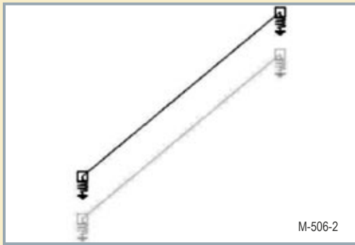
FIGURE 2: Paper cone mode shape at f_0 = 30\text{Hz} , cone mass = 25g, total effective mechanical moving mass = 49g, cone thickness = 0.8mm.
