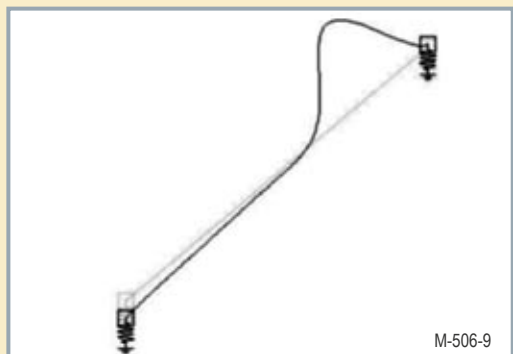
FIGURE 9: Anodized magnesium cone mode shape at f_1 = 1.56\text{kHz} , modal damping = 0.004.
