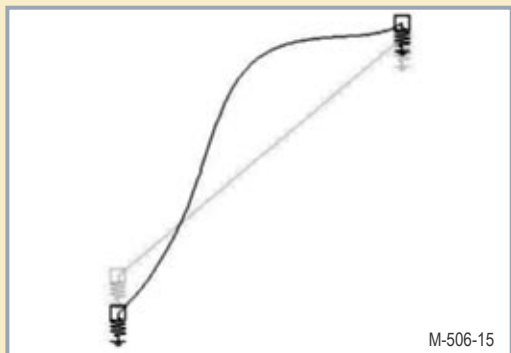
FIGURE 15: Composite cone mode shape at f_1 = 1.75kHz, modal damp- ing = 0.018.
