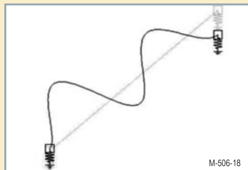
FIGURE 18: Composite cone mode shape at f_4 = 4.00kHz, modal damp- ing = 0.024.
