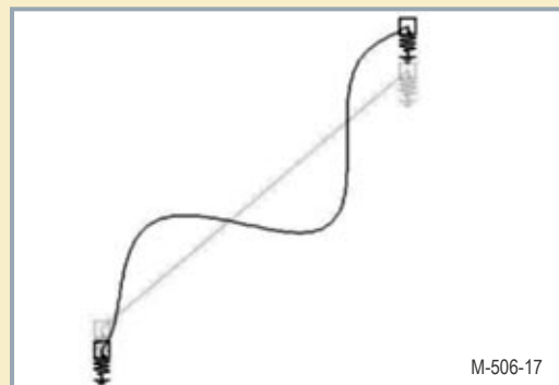
FIGURE 17: Composite cone mode shape at f_3 = 3.10kHz, modal damp- ing = 0.020.
