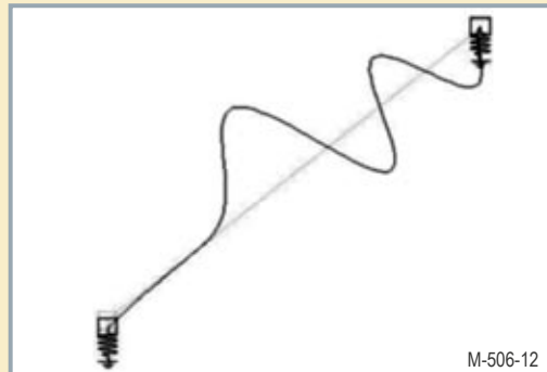
FIGURE 12: Anodized magnesium cone mode shape at f_4 = 2.15\text{kHz} , modal damping = 0.005.
