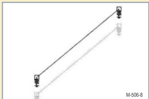
FIGURE 8: Anodized magnesium cone mode shape at f_0 = 30\text{Hz} , cone mass = 25g, total effective mechanical moving mass = 49g, cone thickness = 0.3mm.
