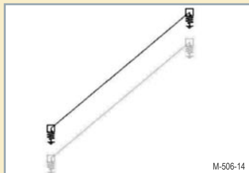
FIGURE 14: Composite cone mode shape at f_0 = 30\text{Hz} , cone mass = 25g, total effective mechanical moving mass = 49g, cone thickness = 2.2mm.
