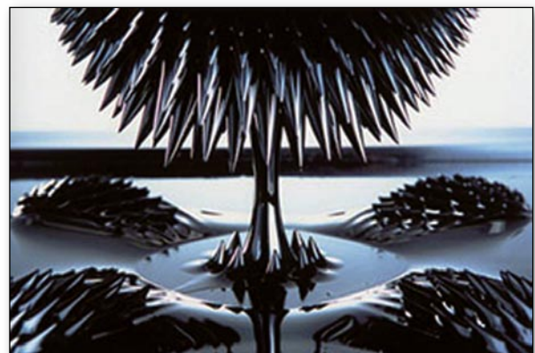
PHOTO 2: Ferrofluid responds to an applied magnetic field.
