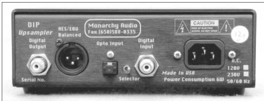
PHOTO 2: Rear panel of the DIP Upsampler. S/PDIF and Toslink inputs are included, plus S/PDIF and AES/EBU outputs. Input switching is done mechanically, with the rear panel selector switch in the center.
