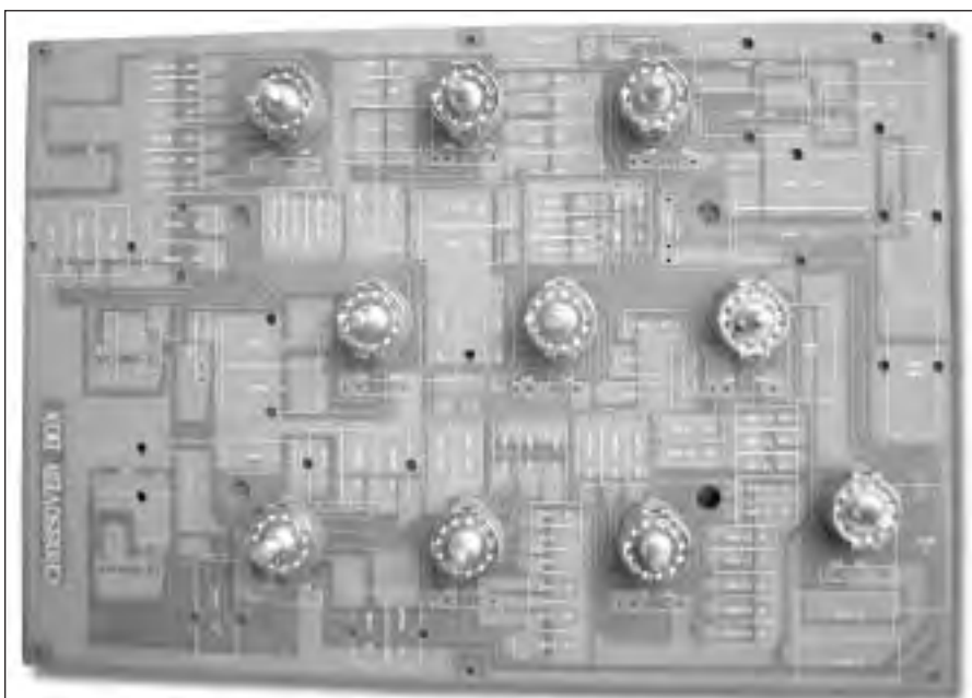
PHOTO 1: VCB-100 printed circuit board with rotary switches installed (courtesy of Vidsonix Corp.).
