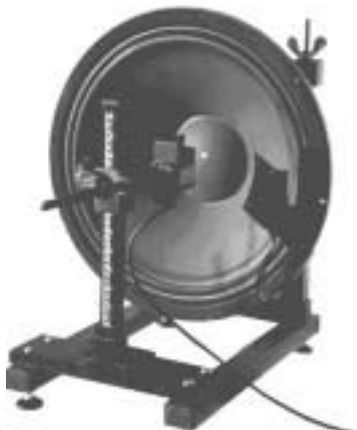
PHOTO 13: A driver mounting stand with laser mount allows diaphragm position information to be collected and sent to the Distortion Analyzer 1.
