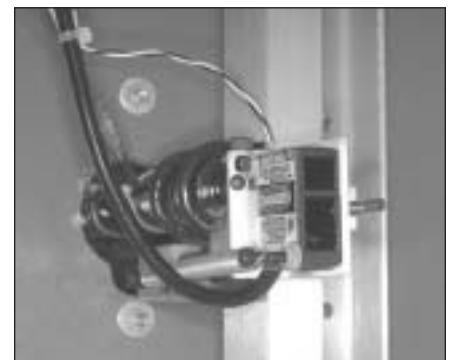
PHOTO 6: The internal laser determines the precise position of the rear of the motor structure.
