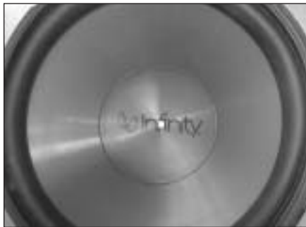
PHOTO 3: A reflective mark placed in the center of the dust cap provides a reference spot for the front measuring laser.
