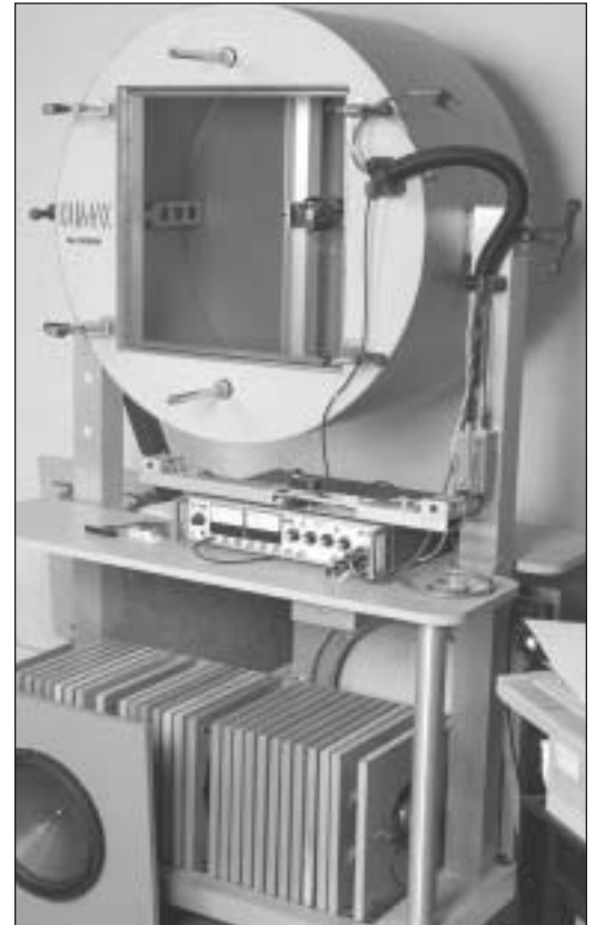
PHOTO 1: The measurement part of DUMAX. Note the ability to rotate the test chamber.
