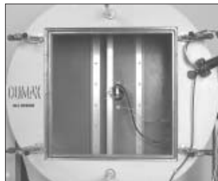
PHOTO 5: A frame inside the test chamber mounts the internal laser.
