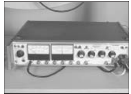
PHOTO 9: The constant-current amplifier provides drive signals, both AC and DC to the voice coil of the driver being tested.
