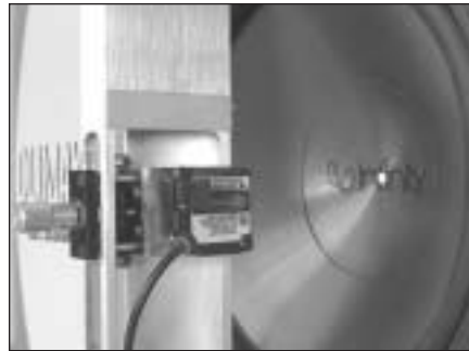
PHOTO 8: The external laser determines the precise position of the dust cap and, therefore, the diaphragm position.
