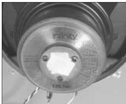
PHOTO 4: A plate with a reflective mark placed in the center of the magnet structure provides a reference spot for the rear measuring laser.
