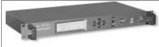
PHOTO 12: The Klippel Distortion Analyzer 1 is the heart of the various modules that make up the Klippel system.
