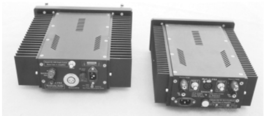
PHOTO 2: Rear views of the amplifiers. The SE-100 Delux is a monoblock. You can configure the SM-70 as a stereo amp or bridged monoblock.
