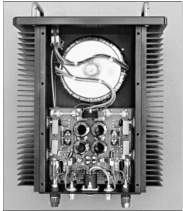
PHOTO 4: Inside the SM-70. Gain is provided by a dual op amp using the conventional feedback technique. The output stage is operated in a zero-feedback, open-loop configuration.
