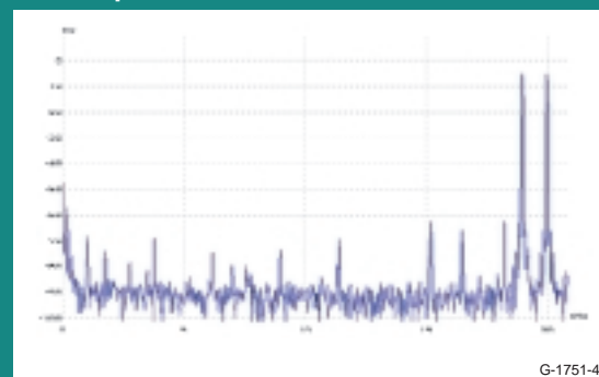
FIGURE 4: Spectrum of 19kHz + 20kHz intermodulation signal.
