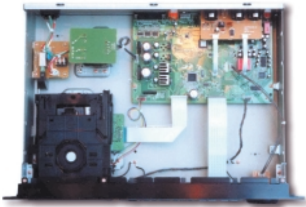
PHOTO 3: Inside the PMD340. The high-performance mechanism incorporates a heavy-duty laser pickup, designed for the demands of the professional user. All ICs on the main PC board are surface-mount devices.
