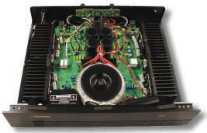
PHOTO 3: HCA-1000A interior view.
