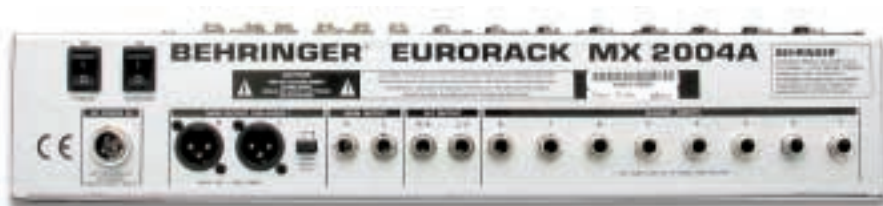
PHOTO 3: Behringer MX2004A rear panel. The XLR main outputs can be switched from line to mike level. Channel inserts for the eight mono inputs, 1/4" main outputs, and the Alt 3 and 4 outputs are on the rear panel.
