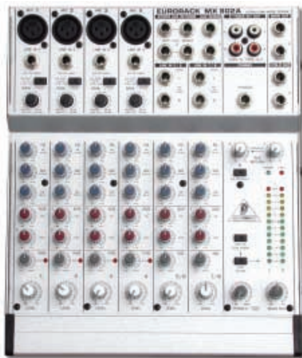
PHOTO 1: Behringer MX802A mixer. The compact design still offers a wide array of features and excellent performance. All audio input and output connectors are on the mixer top plate, as shown.
