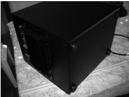
PHOTO 5: Amplifier mounted, and feet attached to the cabinet.
