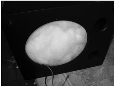
PHOTO 8: The fully stuffed cabinet, ready for mounting the woofer.
