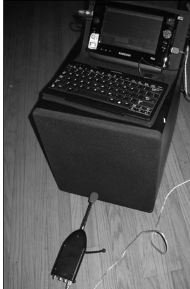
PHOTO 11: Measurement setup, showing the subwoofer, the Ivie Type II microphone, inserted in the IE45 jacket, and connected to an ultra mobile PC running the IE45 RTA software.
