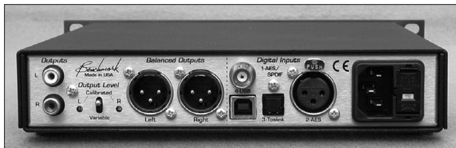
PHOTO 3: Rear view of the Benchmark DAC. S/PDIF, AES/EBU, and Toslink optical inputs are provided, along with a USB connection. Balanced and unbalanced analog outputs are also included.
