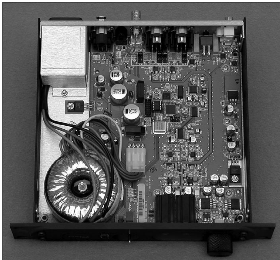
PHOTO 2: Inside the DAC1 USB. State-of-the-art digital chips are used, including Analog Devices AD1896 Sample Rate Converter and AD1853 D/A converter. Construction quality is excellent.
