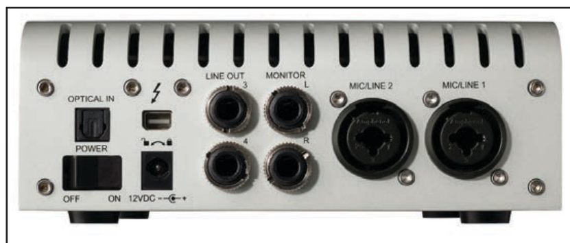
Apollo Twin offers two microphone inputs and two analog line inputs, one Hi-Z instrument input, two analog line outputs (independent mix buses) and two analog monitor outputs, headphone output, TOSLINK optical (ADAT or S/PDIF, selectable) and one Thunderbolt port (Thunderbolt 2). It also has a bayonet-style locking connector to prevent accidental disconnection of the included wall wart power supply.
