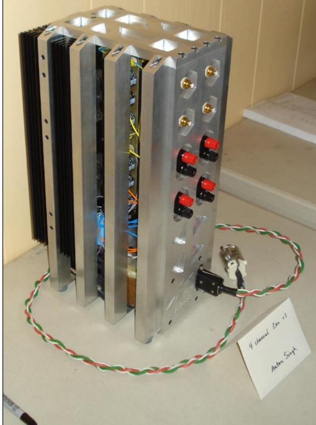
PHOTO 2: Elaborate CNC-based amplifier enclosure design.
