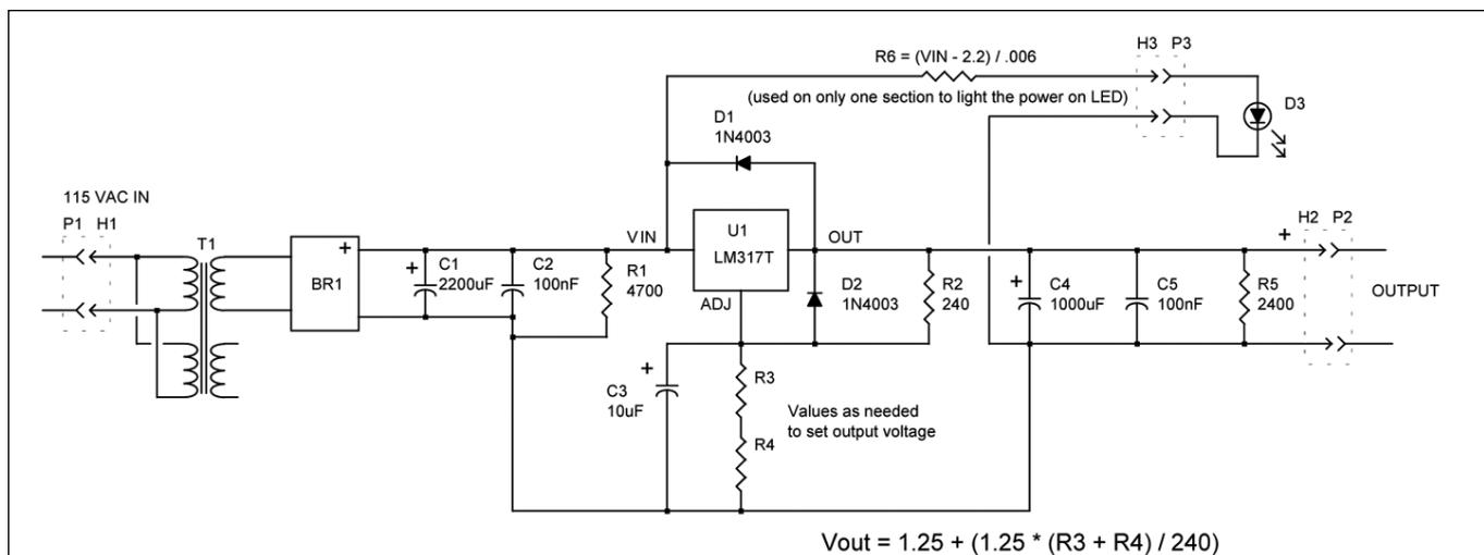
One section of the Multiple "Wall-Wart" power supply.
