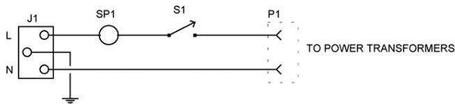
FIGURE 1: Multiple “wall-wart” power supply circuit diagram.
