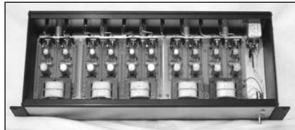
**PHOTO 1:** Multiple wall-wart power supply inside view. The inrush current limiter, SP1, is directly wired to the fused, IEC AC power input connector.
