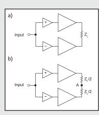
Figure 1: Bridge two amplifiers to make a single amplifier with higher voltage swing capability. The basic bridging topology is shown (a). The load impedance on the output of each amplifier in the bridge is half that of the load driven by a single amplifier (b).
