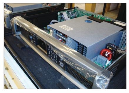
Photo 4: This isn't a top view of the interior; it's a bottom view! Note the inverted construction, which QSC uses to avoid dust collecting on the circuitry and heatsinks.
