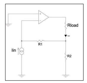
Figure 4: Transimpedance feedback gives rise to a transadmittance amplifier or a voltage-controlled current source (VCCS).
