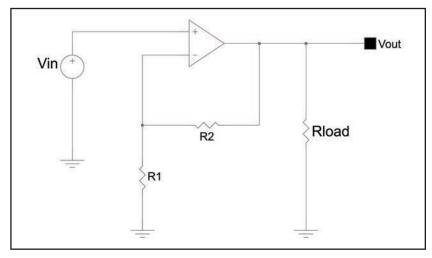
Figure 5: Voltage feedback gives rise to a voltage amplifier or a voltage-controlled voltage source (VCVS).
