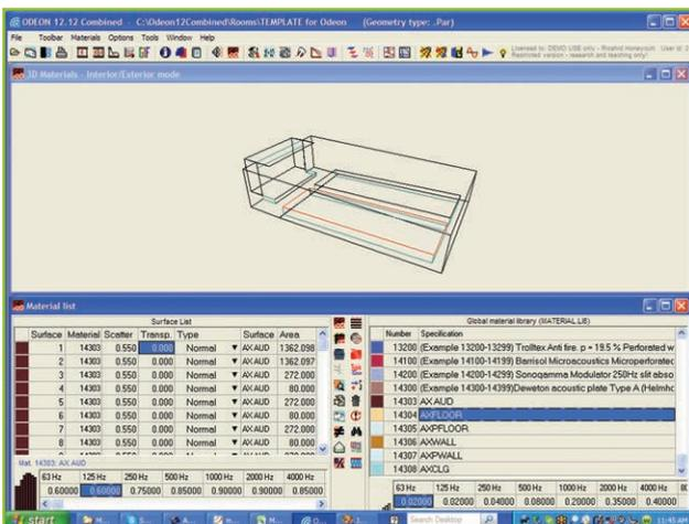
Photo 1: The material list is used to assign materials.
