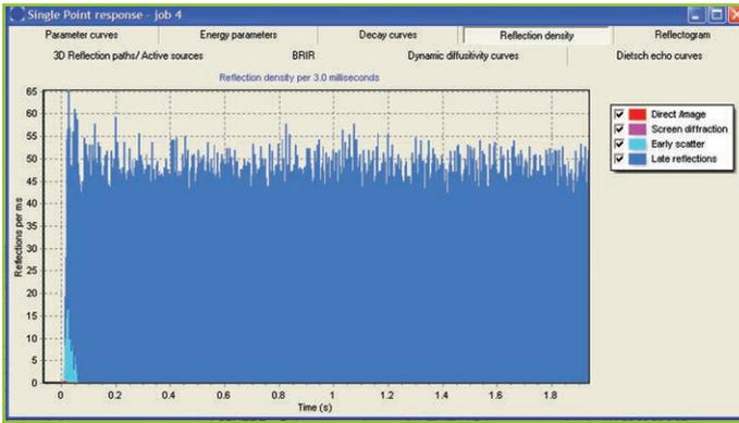
Photo 9: The reflection density plot shows the number of reflections per 3 ms plotted vs. times.
