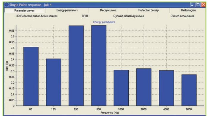
Photo 6: This single-point response shows EDT vs. frequency.
