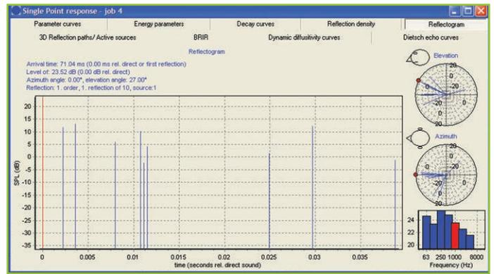
Photo 10: The reflectogram shows individual reflection arrival times.
